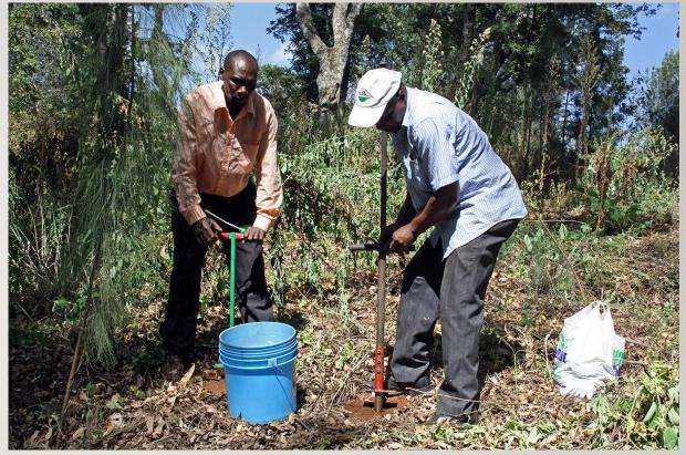
training simple methods of testing the structure of the soil
